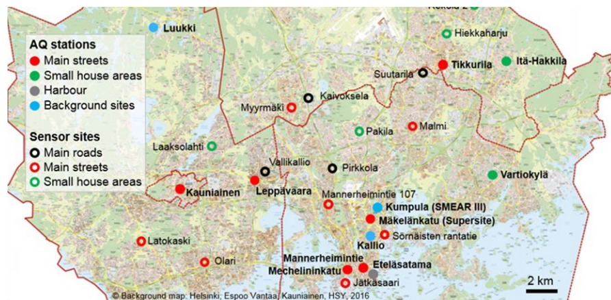
Figure 1 An example of a complementary air quality sensor network. Full circles represent the fixed reference stations, open circles the complementary sensor sites. Different colors indicate different location types. (Source: Helsinki Metropolitan Air Quality Testbed HAQT project)
