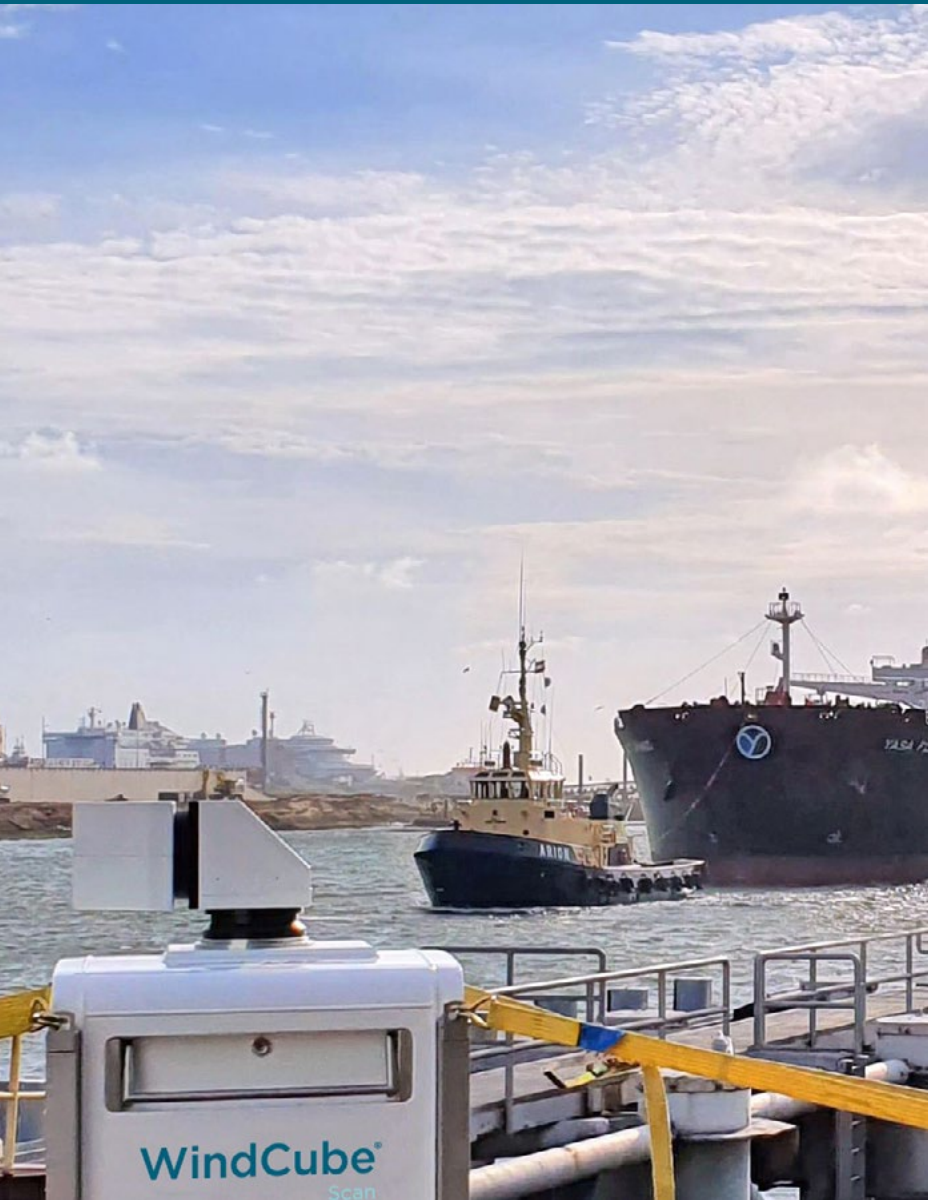
WindCube scanning lidar measuring wind loads on ports
